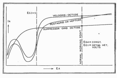
would stop oscillating.) Both groups have the common feature of having a second space charge in which (or close to which) a second control grid operates. The second control grid operates just as Fig. 10.—General characteristics of mixers in group a; note the higher anode impedance of the octodes.
