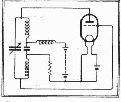
Fig. 10.—The Franklin circuit has a close family resemblance to the Hartley.
