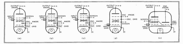
Fig. 9.— Showing relative potentials and functions of pentagrids (heptodes), suppressor grid octodes, velogrid octodes and hexodes. Shaded areas indicate space charges; the normal cathode space charge occupies the area nearest the cathode, while the area between the first positive screening grid and the second negative control grid comprises the virtual cathode space charge.
