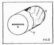
The outside cylinder has a slot at one end and a viewing screen at the other.
