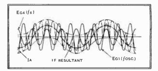
varying. As the anode current depends on the mutual conductance of the second control grid to anode system, which, deriving its electrons from the virtual cathode, is itself a function of the first control grid voltage, it follows that
