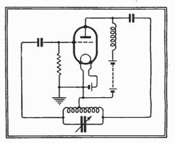
Fig. 5.-The parallel-fed arrangement.
