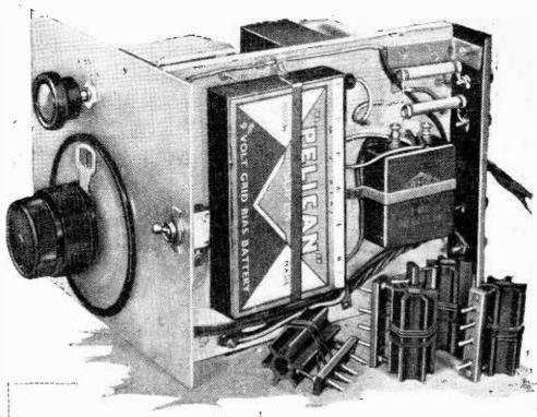
The grid battery, telephone RF chokes, condenser C8, filament and HT wiring are all accommodated below the baseboard.
