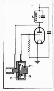
Method of mounting a piezo-electric crystal to "wobble" electric crystal to "wobble" the frequency of a master oscillator stage.
