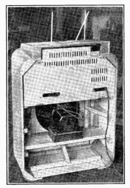
Testing an experimental layout in one of the latest console cabinets for heat distribution. The thermometers indicate the temperature in the vicinity of the oscillator coils, the gang condenser, the electrolytic smoothing condensers and the mains transformer.
