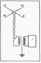
Aerial designed for efficient reception over a wide band of short-waves.
