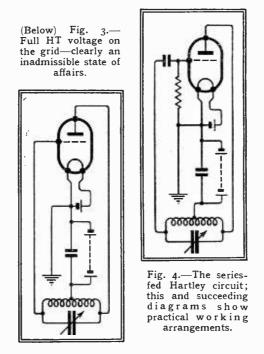
coil between cathode or filament and grid is in the right direction to release across the other part of the coil an amplified voltage that boosts the original oscillation. And so it grows larger and larger until the valve is unable to supply it with enough power to make it grow any more.
