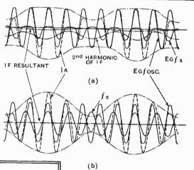
Fig. 2.—Diagram (a) shows additive mixing in grid-rectifying 1st detector; no beat-frequency is produced by additive mixing when rectification is absent as in diagram (b).
