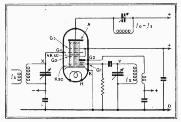
other of the octodes would become the final mixer valve. However, there was one further serious trouble, and this only really came into prominence in 1935-36, when short-wave reception was being asked for in receiving sets; this trouble, as shown in Fig. 12, is due to a falling-off in conversion conductance towards the shorter wavelengths.
