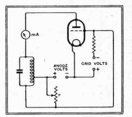
Fig. 12.—A simple form of valve tester, giving direct readings of mutual conductance, based on the information given on the curve sheet, Fig. 11.
