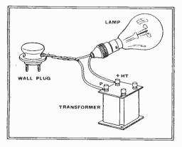
Fig. 1.— Desperate ills call for desperate remedies ; illustrating a scheme that may possibly restore, if only temporarily, a defective transformer to usefulness. or two, three or four times in rapid succession.
