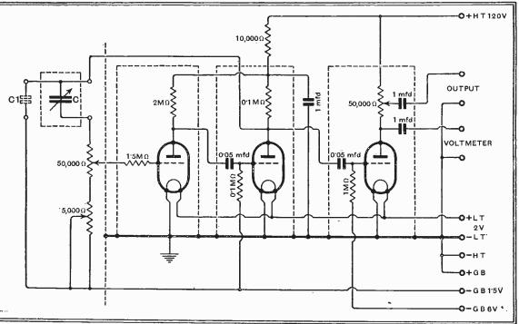
Fig. 3.-Circuit of a practical oscillator; the extra valve provides isolation between the output terminals and the oscillator proper.
