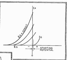
Fig. 3.—The starting potential in early valves was generally in the positive region of grid potentials.
