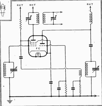
Fig. 8.--Cathode-coupled circuit with triode-pentode valve.
