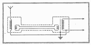
Fig. 1.-Basic anti-interference aerial circuit.
