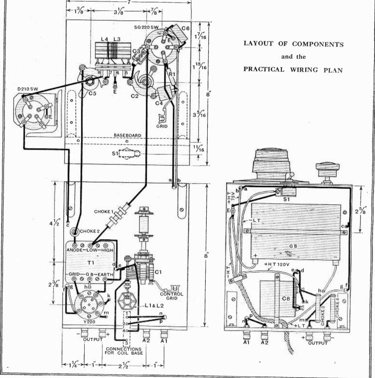
It is essential that everything be made rigid and vibrationless otherwise trouble will be experienced with "wobble " on the received signals. For this reason the panel should be at least 1/16th inch thick and it can be made of aluminium, copper
