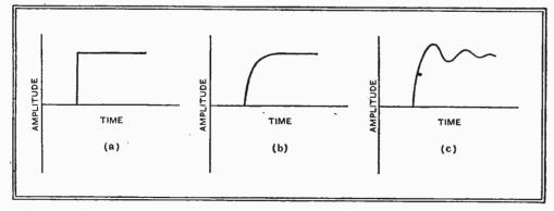
Fig. 25.—A sudden change of voltage such as that shown at (a) will be distorted in the manner depicted at (b) by an amplifier with a limited high-frequency response. With an amplifier of the type of Fig. 26, however, the output voltage may be like that of (c) if the values of components are not properly related.
