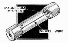
Sensitive to small sustained rises of current, "Mag-Nickel " the "Mag-Nickel" fuse is, nevertheless, unaffected by the surges which occur when the receiver is first switched on.
