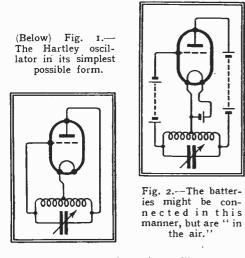
larity of the Hartley; it oscillates very freely; it is simple; and it is easy to understand and to calculate. Against these good points there is the disadvantage that ordinarily both terminals of the tuning condenser are "live"—a feature that may rule it out from such applications as a gang-tuned superhet. However, in some of its forms this difficulty is avoided.
