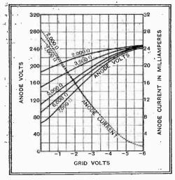
Fig. 31.—Dynamic grid volts—anode volts curves of the TSP4 are given here.
