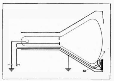
Automatic voltage cut-out for cathode-ray tubes.
