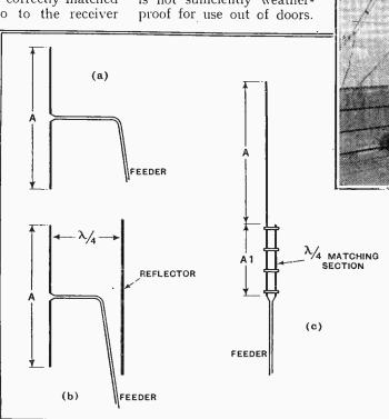
Fig. 2.—The same three aerials as shown in Fig. 1, but here depicted in theoretical form.
