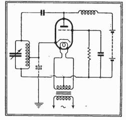
Fig. 9.—The filament choke may be avoided by using an indirectly heated valve.
