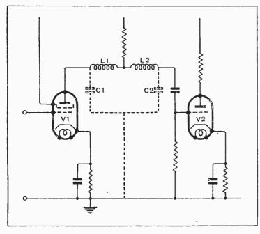
Circuit for amplifier with wide-band frequency response
