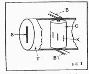
Assembly of the two cylinders in a television scanning system.
