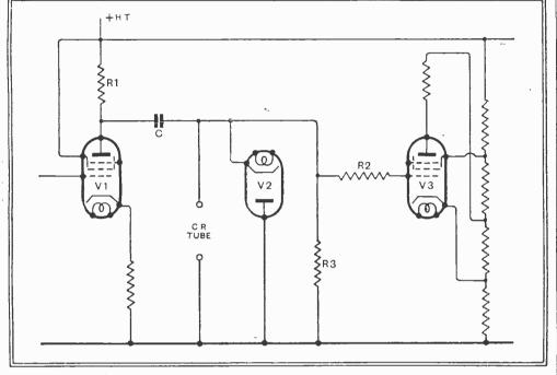
Fig. 24 .-- In this circuit the DC component is lost because of the condenser C, but is restored This arrangement is quite practicable and gives very good artificially by the diode V2. synchronising.
