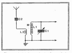
Fig. 2.—Aerial input circuit of a typical receiver ; there is no standardisation of the various constants.
