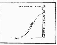
Fig. 15.—Distribution of electrons in the virtual cathode space charge as a function of the voltage on the first grid.
