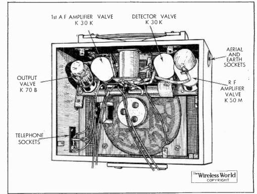
A compact receiver chassis leaves ample space for batteries of standard capacity. The frame aerial windings are incorporated in the sides of the cabinet.
