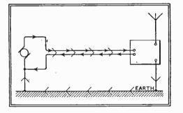
Fig. 1.—The passage of interfering impulses along supply leads.
